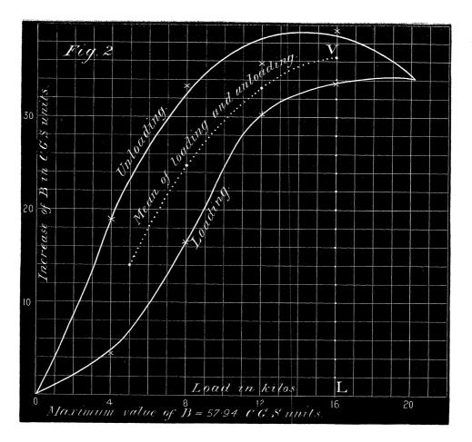
loading and unloading at each stage probably represent what would be the values of A and B if there were no such lagging. In the figs. 1 and 2, which supplement Table XXIII., the *dotted* curves show the relations which exist between the changes of these *mean* values and change of load. The values of both A and B increase with the load until the latter reaches 16 kilos.; further increase of load then causes decrease of A and B.\*
